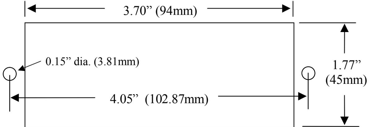
**Figure - 4. Panel Cutout and mounting hole dimensions**
