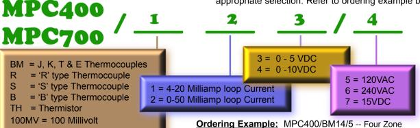
**Ordering Example:** MPC400/BM14/5 -- Four Zone Controller with J,K,T & E Thermocouple, 4-20ma and 0-10vdc inputs and 120vac Power.
